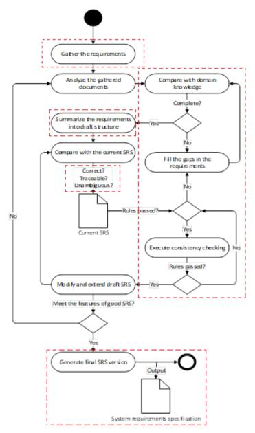
Fig. 12 Upgraded requirements analysis process
