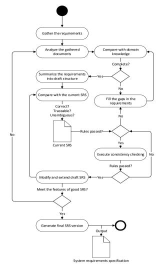
Fig. 4. Upgraded requirements analysis process
