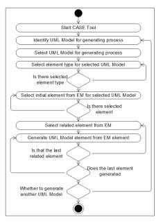
Fig. 3. Transformation Algorithm of EM based UML model generation process
