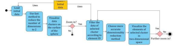
Figure 1. Multi-level method for big data visualisation
